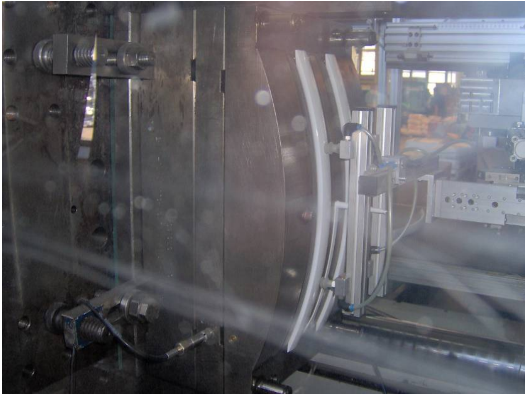
Picture 8. Presentation of the two oven grips SIGMA which are extracted simultaneously from the mold
